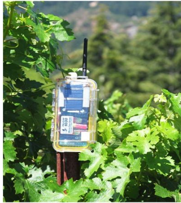
Figure 1: DOT – Wireless Sensor Network Device Deliberate to be the Estimated Size of Area
